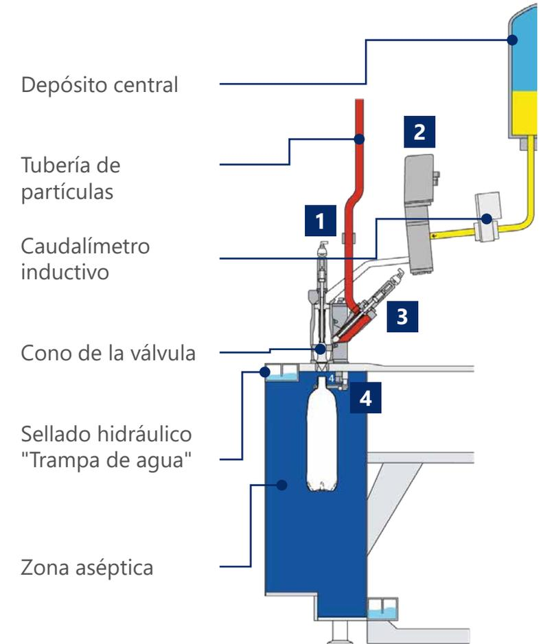
VFJ-D: Volumetric filling, Flow meter, full Jet, Double filling valve | PFR: Proportional Flow Regulator
