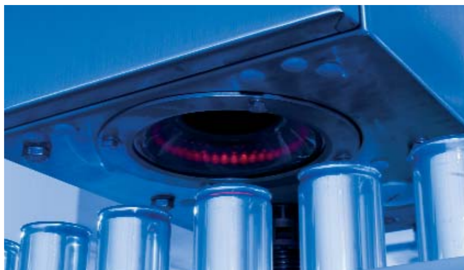
The Cantronic D checks up to 120,000 beverage cans or food tins per hour for contaminants and grooves.
