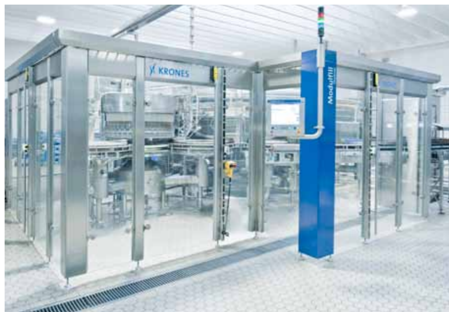
The filler's modular design makes it easy to synchronise into a bloc arrangement with other machines.
