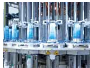
The new Sleevematic ES labeller handles highly elastic film sleeves.
