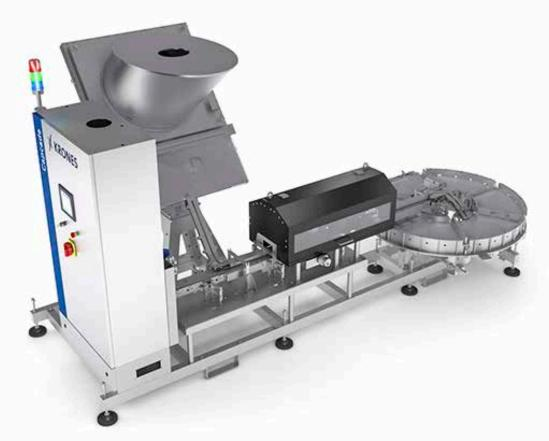
Note: Cap sorter with Checkmat inspection system and Accucap cap buffer system is installed on a separate platform
