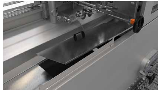
The tanks are accessible both from above and from the side.
