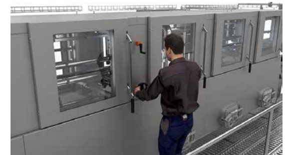
Both the height and the width of the guide can be easily adjusted from the outside.
