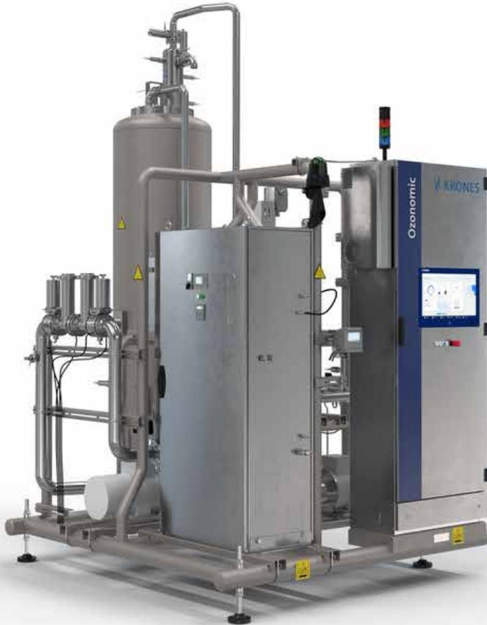
The Ozonomic operates on the principle of "still electrical discharging". In this principle, the oxygen flows through the ozone generator module. The high-voltage electrodes contained there discharge electrical energy, which causes oxygen molecules ( $O_2$ ) to split and ozone molecules ( $O_3$ ) to form.
