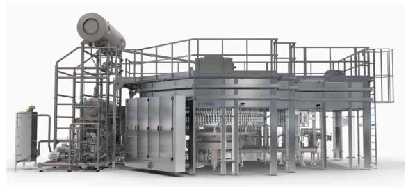
With the Modulfill VFS-M, the "M" stands for "Mixer" – which is directly connected to the filler. The product is directly fed via the raised carbonation tank into the manifold. The conventional filler bowl is no longer required. Thanks to optimised interfaces, the number of components is also reduced and thus not only the footprint is reduced, but also the running operating costs.
