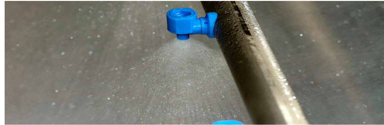
Spraying nozzles in the LinaFlex
