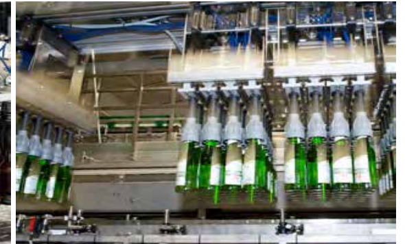
One-dimensional, flexible gripper unit for precise insertion into packs
