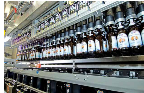
Orientation gripper unit for swing-stopper bottles
