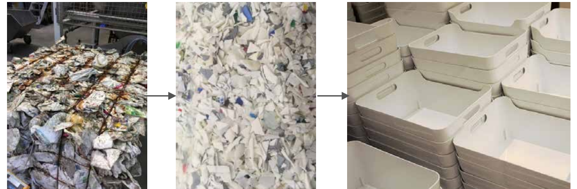
Creation of clear and odourless PO flakes
