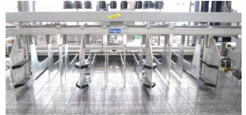
Gripper unit handling parts (packer) with insertion frame, bottle guide plates and vibrator
