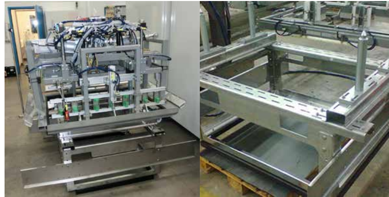
Example: Head support frame for gripper unit storage
