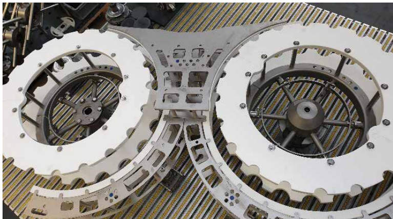
Curbed infeed/discharge guide with starwheels
