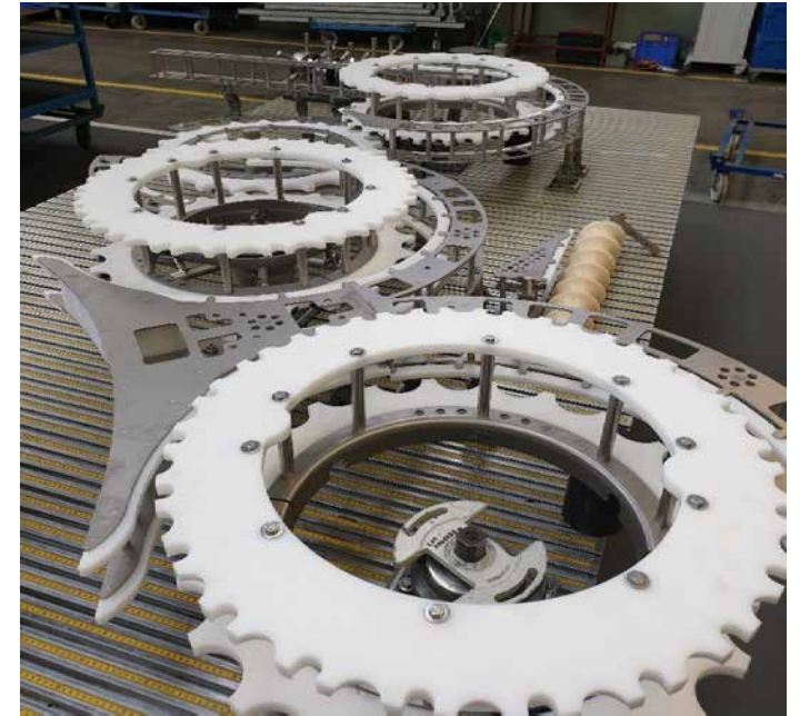
Curved infeed and discharge guide with starwheels
