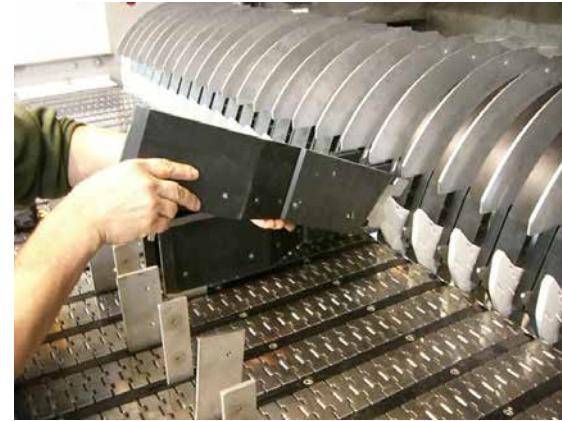
The bottle guides can be easily replaced during product change-over
